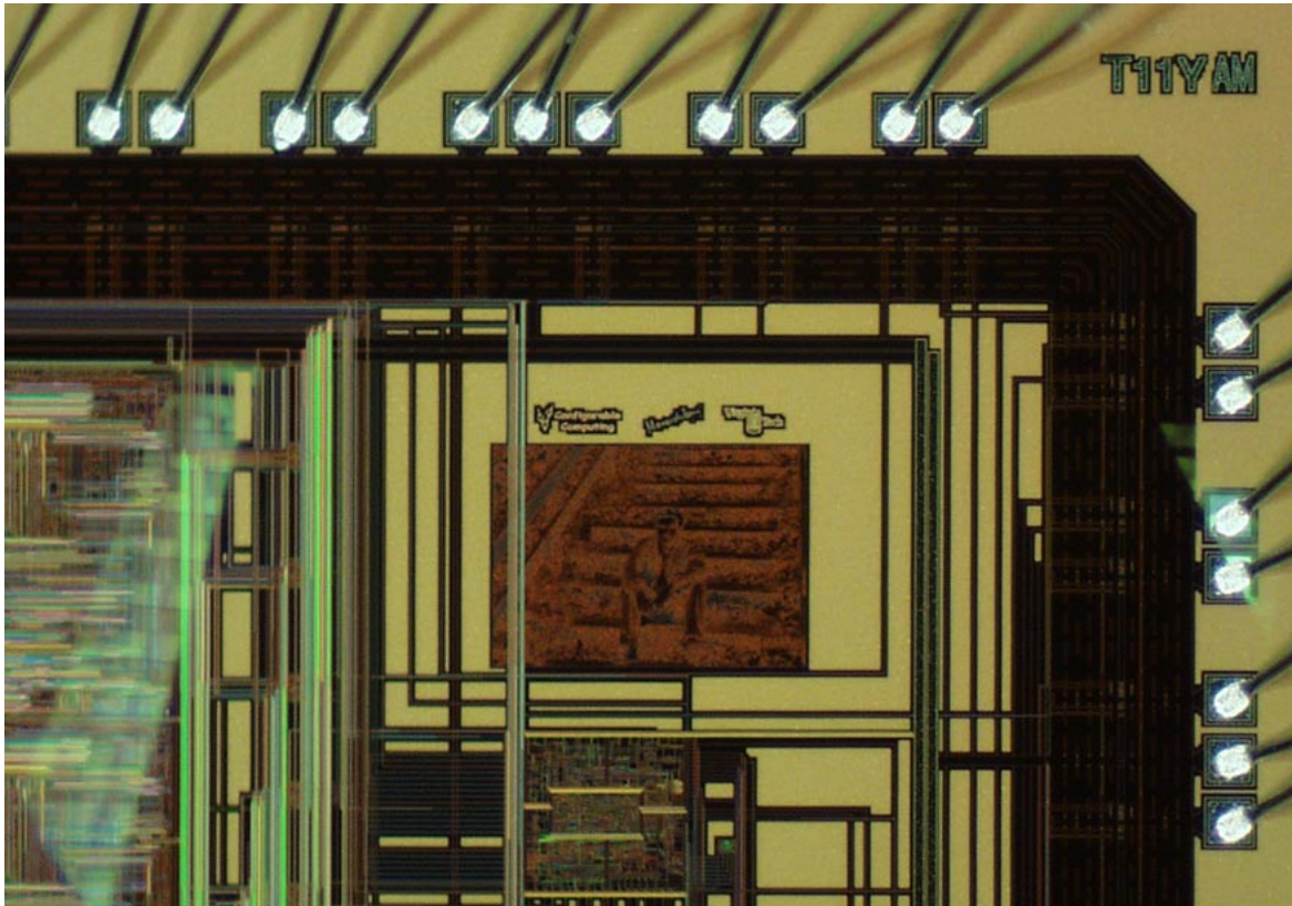
Figure F-2 Photograph and logos embedded in Stallion using the p2m tool
