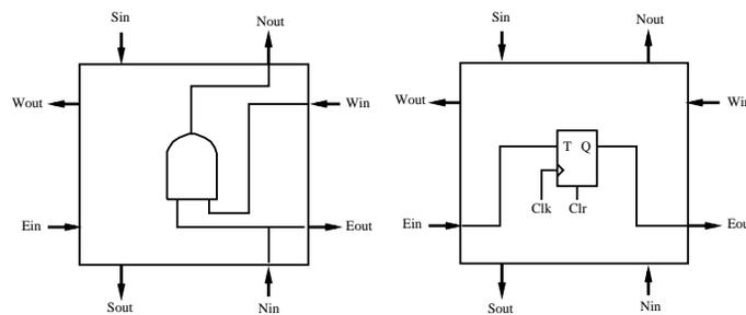
**Fig. 4.** The carry and toggle flip flop cell definitions.
