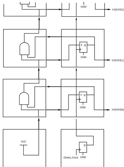
Fig. 6. The relative locations of cells in the counter.
