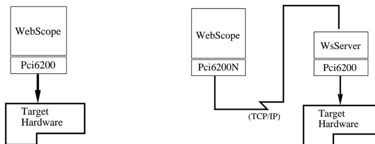
**Fig. 2.** Local and remote access to the target hardware.
