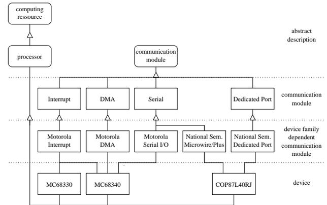
**Figure 5. Object oriented modeling of processors**
