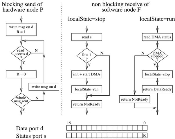
**Figure 7. Interface refinement for channel B**
