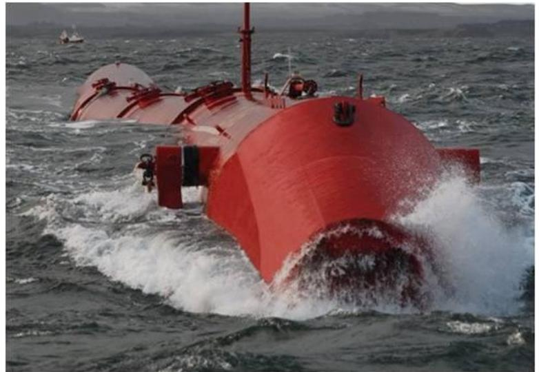
Fig. 2; PELAMIS wave power: creating electricity by the sea.
