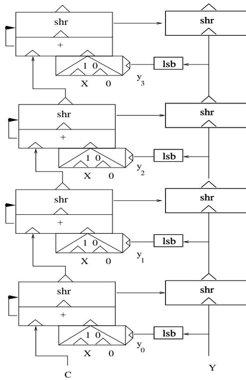
Figure 3: Circuit schema for 4-bit numbers multiplication
