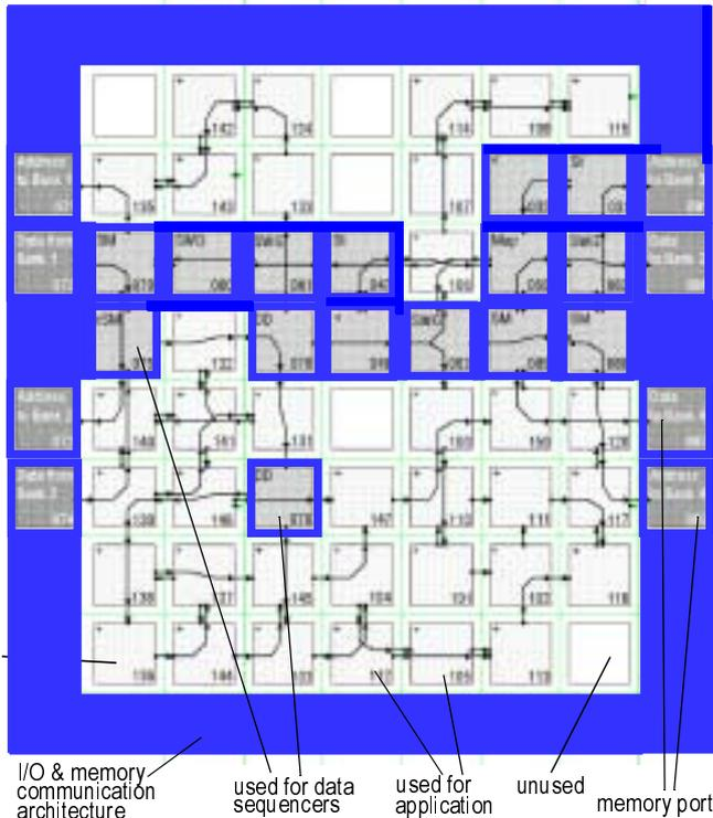
Fig. 5: Mapping application (linear filter) and memory communication architecture (dark background) onto the same KressArray, including the address ports and the data ports to 4 different memory banks (5 of 8 memory port connects are routed through application DPUs).
