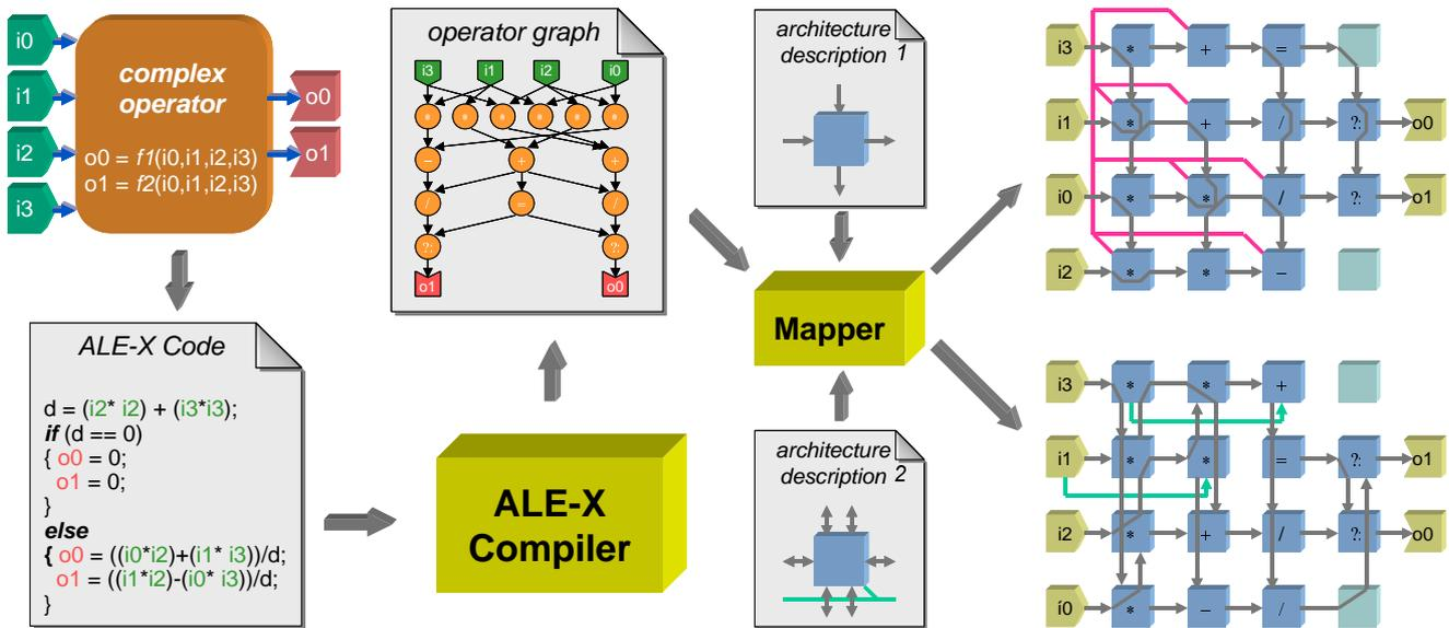
Fig. 10: Simplified example to illustrate platform space exploration (finding an optimized KressArray by KressArray Xplorer [43]).
