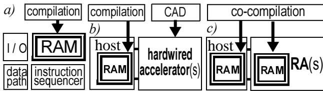
Fig. 12: Computing Platforms: a) “v. Neumann”, b) current, c) emerging.
