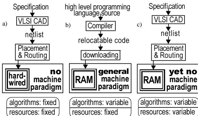
Fig. 9: Synthesis a) hardwired, b) “von Neumann”, c) reconfigurable.
