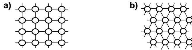
**Figure 3. Possible routing structures of the rDPA chip a) mesh, b) hexagonal array**
